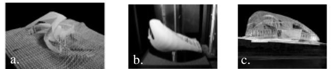
Figure 5 – a. Laser cut frame model; b. RP skin model; c. CAM final model
