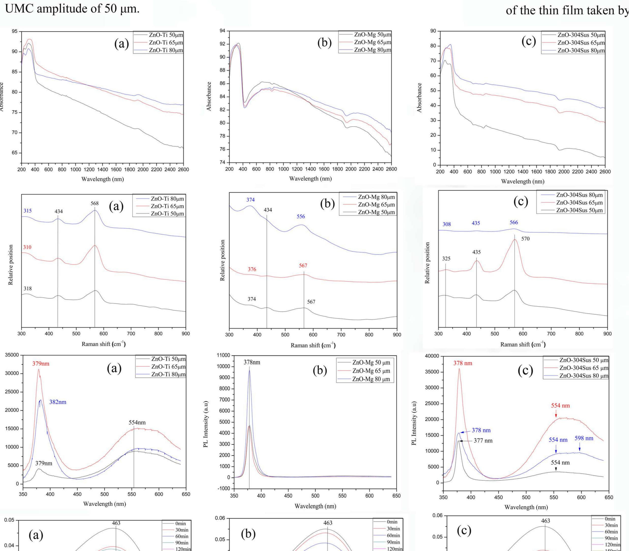
Figure 6. The UV-Vis absorbance spectra of black ZnO thin films on Ti, Mg, and 304Sus substrate with the UMC amplitude of 50 µm, 65 μm, and 80 μm, respectively.
