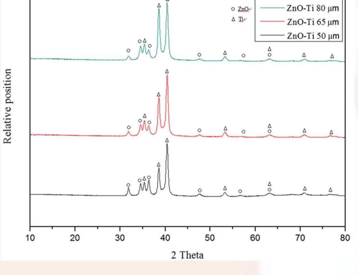
Figure 3. The XRD of black ZnO thin film on Ti substrate with the UMC amplitudes of 50, 65, and 80 μm, respectively.
