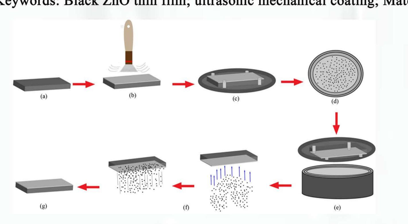
Figure 1. Ultrasonic shot peening process: (a) selecting a suitable substrate; (b) brushing the alcohol and ZnO powder mixed solution on a selected substrate and making it evenly distributed; (c) fixing the substrate with colloidal ZnO on platform; (d) putting stainless steel balls in the holder; (e) covering the platform on the holder; (f) running ultrasonic shot peening; (g) final product.
