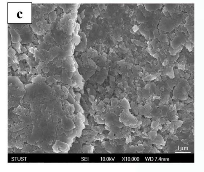
Figure 4. The SEM images of black ZnO thin film on Ti, Mg, and 304Sus substrates with the
