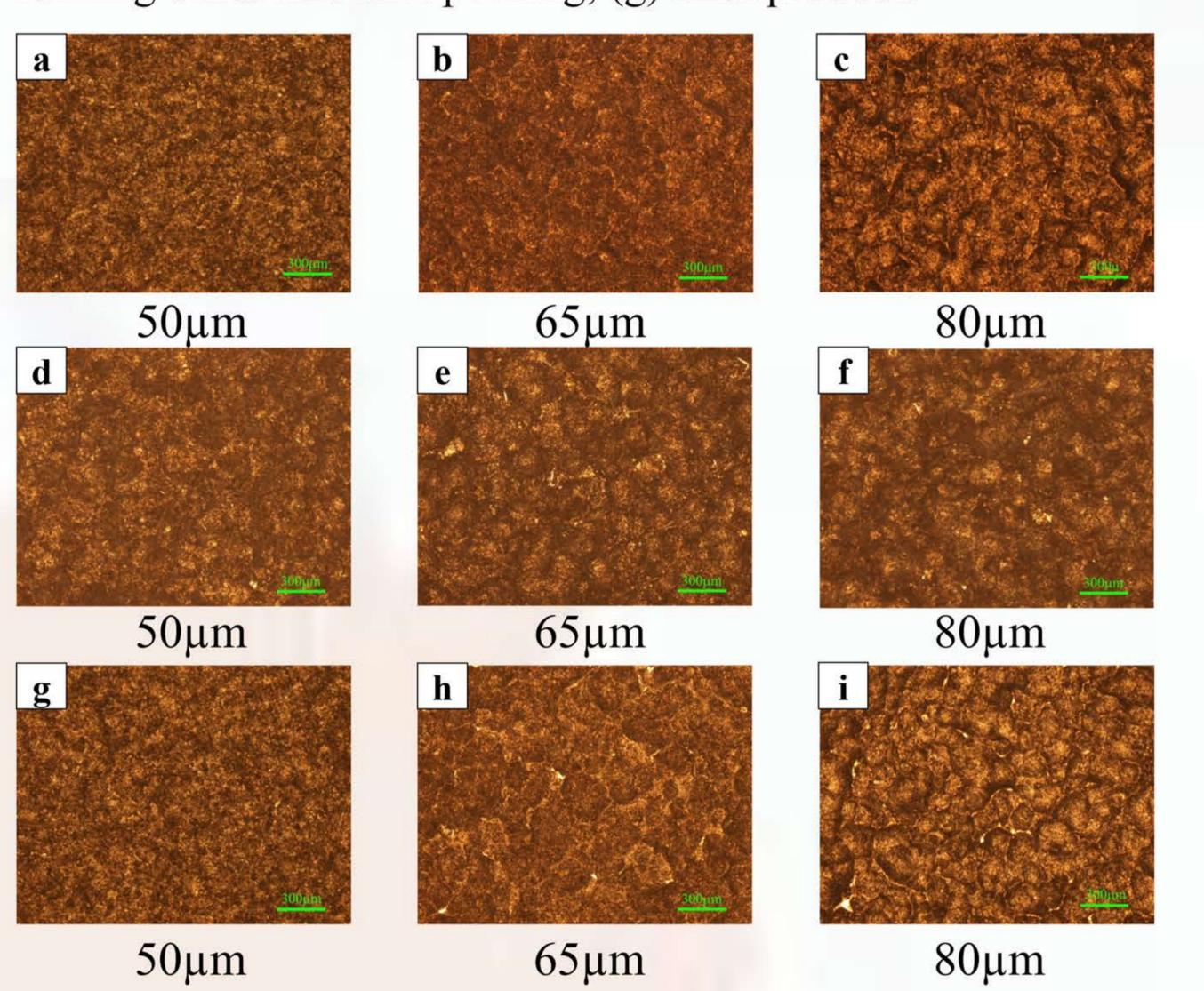
Figure 2. The optical microscopic observations on three different substrates: (a) to (c) for Ti, (d) to (f) for Mg, and (g) to (i) for 304Sus with the UMC amplitudes of 50, 65, and 80 μm, respectively.
