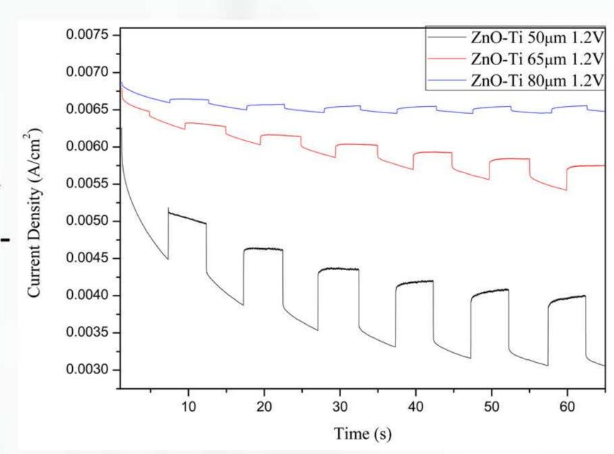
Figure 11. The photoelectrochemistry images of black ZnO thin film on Ti substrate with the UMC amplitudes of 50, 65, and 80 µm, respectively.
