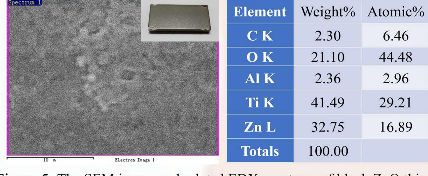
Figure 5. The SEM image and related EDX spectrum of black ZnO thin film on Ti substrate with the UMC amplitude of 50 μm. The inset shows the image of the thin film taken by camera.
