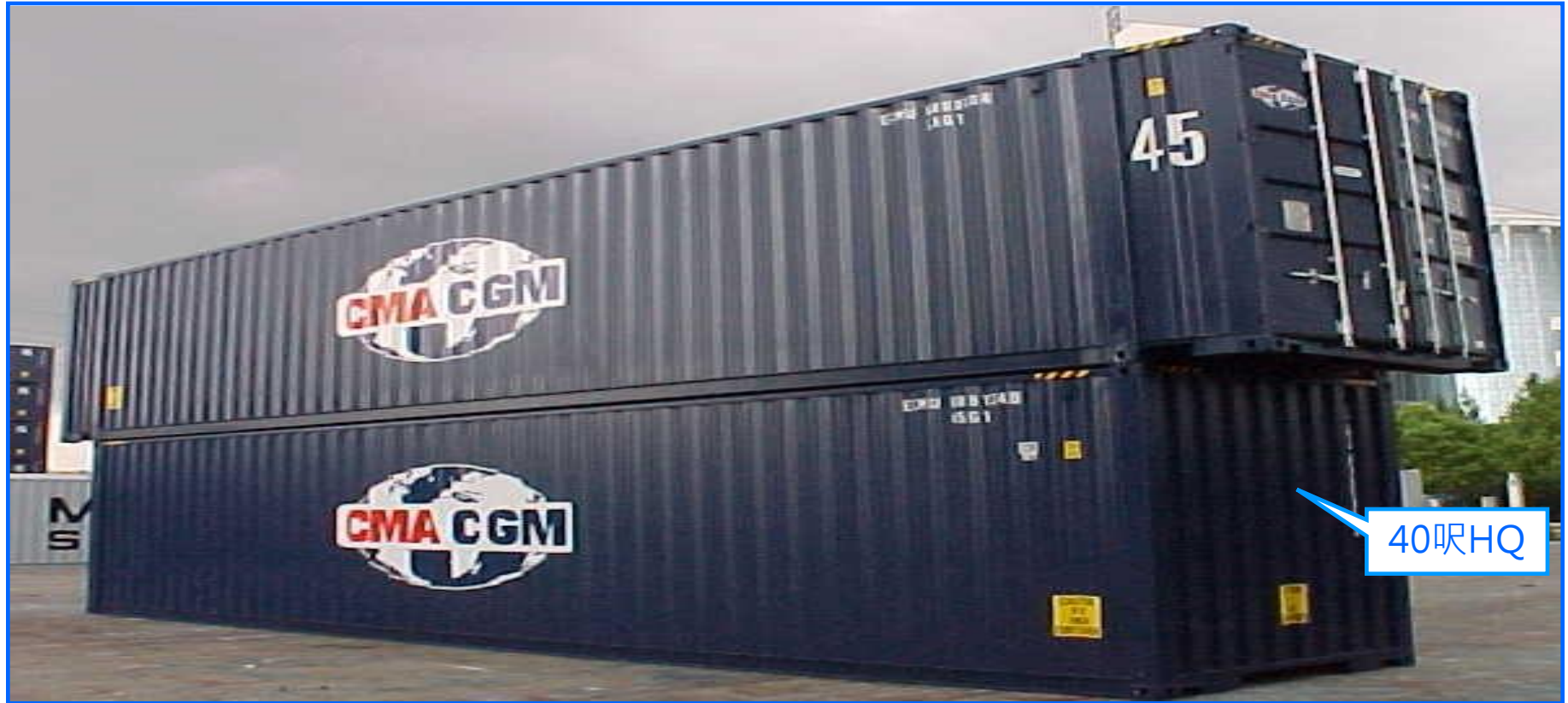
40 呎超高鋼製乾貨貨櫃( 40' Hi-Cube Steel Dry Cargo Container)
